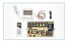
For Cabinet Air Conditioner Sleep function, Auxiliary heating Auto restart, 3 sensors LCD back light display panel Negative ion control Memory and auto restart Outdoor fan controlled independently Interior power indicator Auto / manual air direction control
