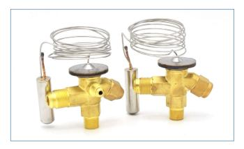
RFKH series thermostatic expansion valves adjust mass flow of refrigerant into the evaporator while controlling the refrigerant's superheat at the evaporator outlet.
